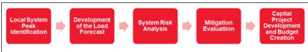
14 FIGURE DCM-D-1 Overview of Load Forecasting Process
